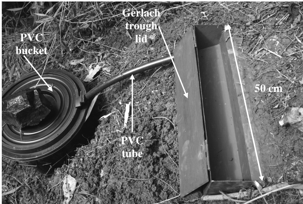
Figure 1. The Gerlach trough system used to collect event surface runoff.
